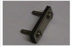
Place plate/valve assembly on upper diffuser assembly. Secure using 10 x 20 SS screws and nylon sealing washers. Locate washers in holes in the port plate and tighten firm enough to seal. NOTE: new screws and diffuser thread should be lubricated with copper grease.
