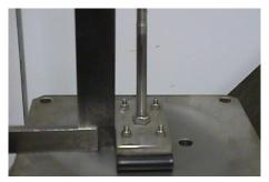
• Put screws through the final clamp bar and push through the clamp bar seal. This must be a tight fit. Place the screws through the remaining holes in peel valve then through the centre of the port plate. Put on lock nut and ensure valve is parallel to the sides of the port plate. Tighten to give a firm grip but do not distort valve rubber.
