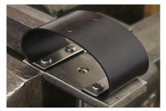
To check place valve down on a flat surface (e.g. port plate) and check that valve sits square with the operating rod at 90° to the plate and both ends square to the operating plate with no tendency of the valve to wrinkle up.
