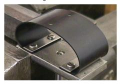
To check place valve down on a flat surface (e.g. port plate) and check that valve sits square with the operating rod at 90° to the plate and both ends square to the operating plate with no tendency of the valve to wrinkle up.
