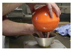
Re-check adjustment by dropping the ball into the cone and noting the gap through the mesh of the diffuser, also check for valve upsetting due to poor alignment.  The completed assembly can now be bolted to the top cap using a separator cap gasket and four copper greased 10 x 33SS screws and spring washers.
