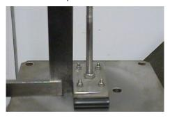
Put screws through the final clamp bar and push through the clamp bar seal. This must be a tight fit. Place the screws through the remaining holes in peel valve then through the centre of the port plate. Put on lock nut and ensure valve is parallel to the sides of the port plate. Tighten to give a firm grip but do not distort valve rubber.
