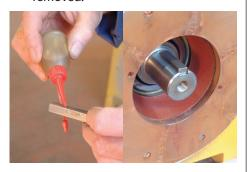
• Lubricate impeller key with oil and fit to shaft.
