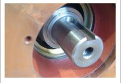
First inspect the lead in chamfer on the pedestal stationary face recess – this should be smooth, clean and rust free
