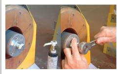
Lubricate the stationary seal recess and lead with a very diluted solution of soft soap. Lubricate the outside of the stationary face assembly with clean water only and using tool 1596131000 push the seal face firmly to the base of the recess. The use of the tool will ensure that the face is fitted square to the shaft axis.
