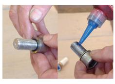
Fit the M16 cap screw with a new Dowty washer and grease the face of the washer. Apply Locktite nutlock 242 to free end of the thread.
