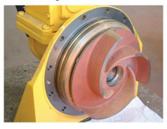
The impeller/seal assembly can now be mounted on the shaft taking great care not to contact the seal face on the shaft or key whilst locating the shaft in the bore. Keep pushing the impeller forward until the seal faces contact.
