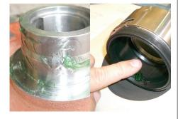
• 'With clean hands' apply soap to the outside of the impeller boss and lead. Lightly soap inside the back of the rubber bellows.
