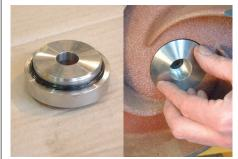
Grease the 'O' ring and fit to impeller collar. Fit collar into impeller.
