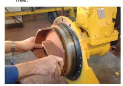
The new or 'cleaned up' impeller should be checked for a tight but sliding fit on the shaft and key.
