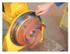
• The front clearance should then be checked and adjusted. Rebuild all further components using new 'O' rings and gaskets. Refill flushing chamber to plug with oil prior to running unit.
