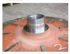
• Lay the impeller blade side down on a firm surface. Lightly oil the bore and keyway.
