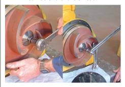
Push impeller back against seal spring and locate and tighten cap screw. Using a 14mm hex socket adaptor torque to 122Nm by jamming the impeller with a wooden block against the drain tap recess in the volute.
