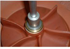
Reassemble rest of pump in accordance with pump manual using new gaskets.
