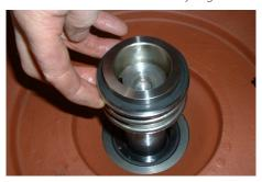
Lubricate the impeller key with Shell Ensis or grease and locate in the key way. Apply Ensis/ grease to the bore and key way of the impeller. Mount the impeller onto the Shaft, and push firmly against the shoulder of the shaft sleeve.
