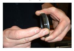
Push it home into the recess ensuring that it is seated square and firmly against the shoulder at the bottom of the recess.
