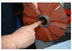
Using a new patched impeller bolt two Belleville washers and an impeller Washer, push the impeller forward compressing the spring of the seal until a torque of: 81.3 Nm for S100 or 108 Nm for S150 + S200 is achieved. Jam the Impeller using a block of wood from the impeller blades to the drain tap recess or cutwater to prevent shaft rotation during this procedure.
