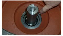
E. The stainless steel seal mounting sleeve must be in good condition. Clean, smooth and free from burrs and scratches.
