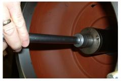
Tighten centre bolt on tool to push face into the housing, when fully home keep tool in place for 10 seconds before removal to allow the rubber to relax into position. Withdraw tool and Inspect for contamination of face and wipe clean if necessary.
