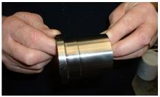
F. The impeller and seal sleeve must be a tight but sliding fit on the shaft.
