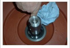
Place seal/ sleeve assembly on the drive shaft being careful not to contact the face on the shaft end, push forward until seal faces contact firmly together.
