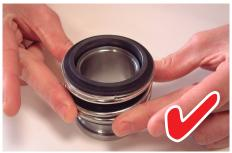
Press on the bottom coil to push home, Do Not apply any pressure or force to the seal face.
