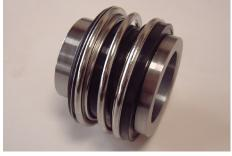
Check that the bellows abuts the shoulder all around the base.
