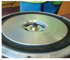
To replace the actuator valve smear the bore with soft soap and ease the new valve rubber into position ensuring that it seats correctly.
