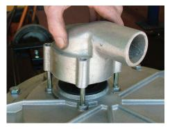
Pull the old valve off the stud head, and discard.
