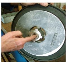
Seat the outside section of the actuator seal in the inner pump body recess by gently tapping with a nonmetallic mallet.
