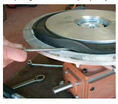
Remove the actuator screw and withdraw the actuator complete with the seal from the drive rod.
