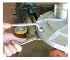
Remove the valve by pulling it off the actuator nut.
