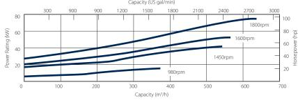
Please note: The above curves cover the complete range and ability of the pump unit. Actual performance will be subject to the engine / motor indicated overleaf and medium pumped.
