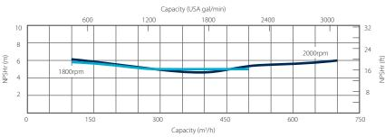
**Please note:** The above curve covers the complete range and ability of the pump unit. Actual performance will be subject to the motor/engine indicated overleaf.
