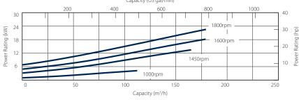
Please note: The above curves cover the complete range and ability of the pump unit. Actual performance will be subject to the engine / motor indicated overleaf and medium pumped.
