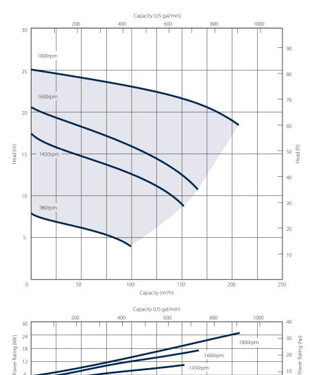
Please note: The above curves cover the complete range and ability of the pump unit. Actual performance will be subject to the engine / motor indicated overleaf and medium pumped.
